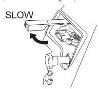
Figure 33. Throttle Lever (Slow Position)
